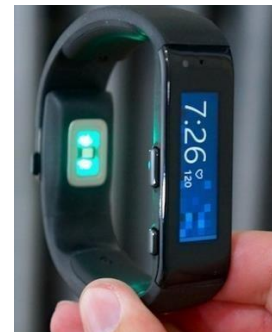
Health Band: Monitoring Heart rate and instantly communicate with smartphone, so doctor can monitor his patients remotely
